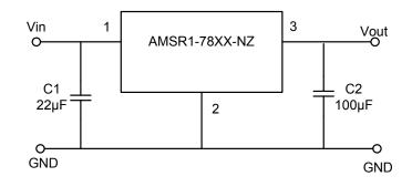
C1: A low ESR capacitor is required to keep the noise of the converter to a minimum. Ceramic capacitors are recommended, but tantalum or electrolytic may be used. Typical value is  $22\mu$ F / 50V. C2: Installation of C2 is recommended but optional. Typical recommended value is  $100\mu$ F / 25V electrolytic. **NOTE: This part is not designed for parallel operation.**
